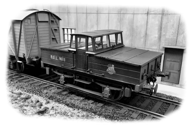
This is an etched brass construction kit based on the battery electric locomotive that worked the Midland's coal depot near West India Dock in Poplar, East London from 1913 to 1964. There was no rail access to the depot the only means of access was by a hydraulic wagon hoist hence the size, height and weight of the loco which had to use the hoist for maintenance or overhauls. A number of similar locos were produced to suite industrial locations.
