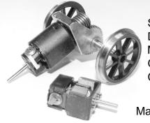
SINGLE AXLE DRIVE USING SMALL MOTOR AND 40:1 GEARBOX FOR ONE OR BOTH AXLES
